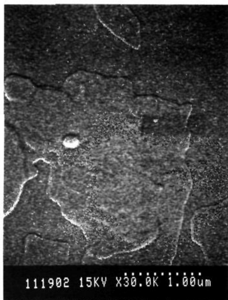
Figure 2. Scanning electron micrograph of the surface of the layered silica-C16TAB composite film. This micrograph was obtained on a Hitachi S-900 scanning electron microscope.
